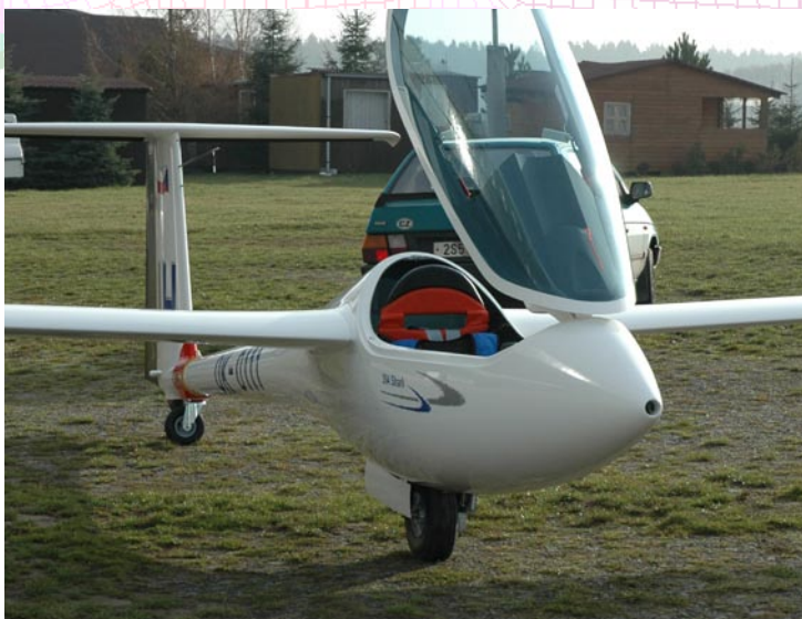
The long travel of the shock absorbing strut provides comfortable landings.
