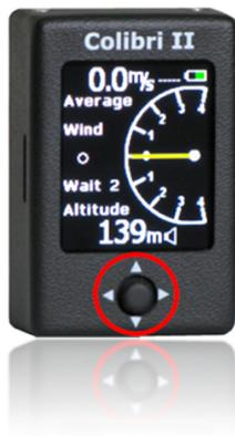
There is one multifunction switch, the **navigation switch**, on the front of the unit that is used to control the Colibri II. The **navigation switch** allows five motions:
