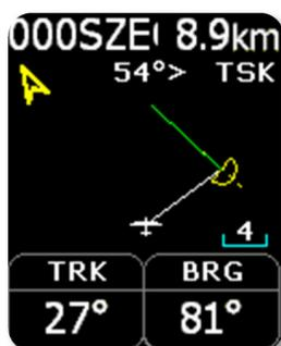
The task page guides the pilot from the start point over turn points and then to the finish line. All points of a task should be included in the unit's internal TP file. The task page provides navigation information to the pilot towards the selected TP from a task. The screen shows the same layout and information as the TP Navigation page and navigation is always orientated track up.
