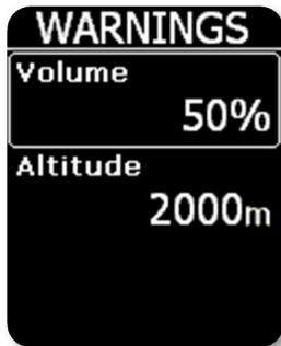
The Colibri II will alert with an audible alarm when a preset altitude, based on QNH settings, is reached. A warning message will also be shown on the screen and the pilot is obliged to acknowledge the warning with the enter button. To turn altitude warning OFF, set altitude to minimum value and next value will be OFF.
