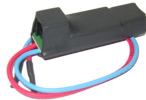
The unit has two plugs. On one side there is a standard USB A connector. Use the included USB cable to connect the Colibri II on this side. On the other side is an RJ45 plug. This plug is a standard IGC 6-pin connector.
