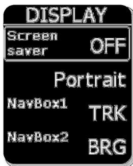
If you activate the screensaver mode, then after the screensaver timeout period, the LCD backlight turns off. Every 10s a message "Screensaver is active!" will appear for one second to show that the unit is functioning. Pressing any key will deactivate screensaver and will also reset its timeout. If you intend to use the unit only as a flight recorder, then using the screensaver mode can extend battery endurance by 3 hours to a total of 10 hours.
