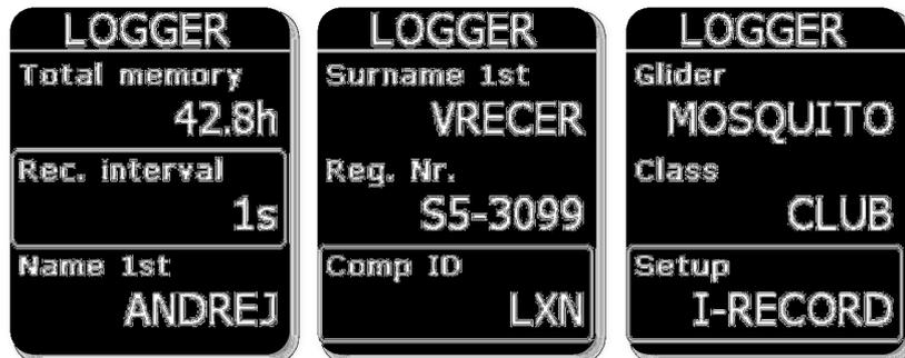
To change the text string, press the enter button and a cursor will appear. Using the up and down button change the letters. The left and right buttons move the cursor position in the text string. **The entered string will end behind the cursor when enter button is pressed.**
