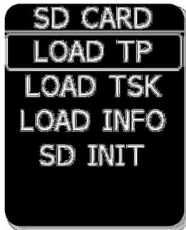
**LOAD TP:** Transfers turn point data from SD to device. Pressing the enter button will show a list of **first 20 \*.cup** formatted files in the LX/TP directory on the card. Select the file of interest and start the transfer with enter.
