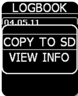
Pressing enter on any flight of the logbook will enable the **Copy to SD** and **View Info** function. Copy to SD will copy the selected flight to the SD card. View Info will show the pilot and glider data.
