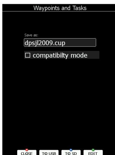
Change the filename if required. Press **TO USB** for saving to the USB stick or press **TO SD** for saving to the SD card. When the compatibility mode flag is checked the file will be saved in DA4 format, which can be used with older LX devices (LX20, Colibri, LX5000, and LX7000).
