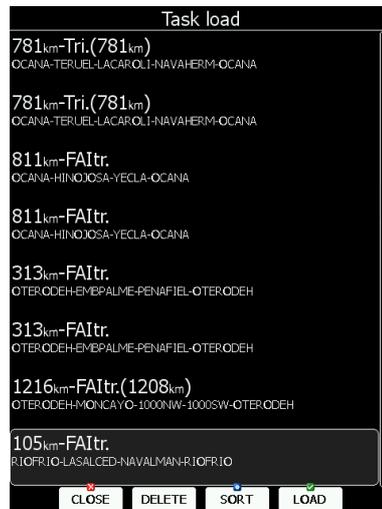
Total task distance, task description and task points are shown for each task stored. Select the desired task by rotating the lower-right knob and press **LOAD**. The task will be loaded into the active task and the task edit dialogue will be opened.
