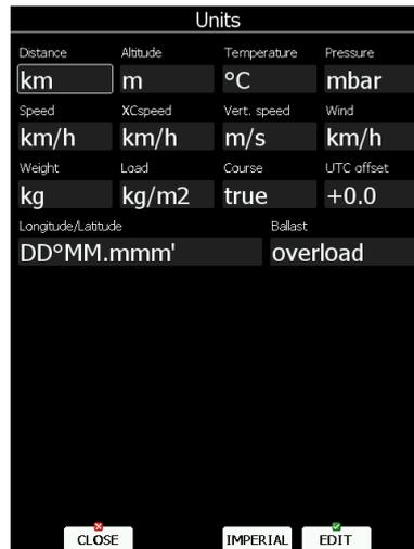
The lower-middle button will toggle all units between imperial and metric units. Glider ballast can be entered as:
