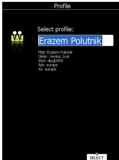
Turn the lower-right knob to select the desired profile if more then one profile is available. For the selected profile the pilot name, glider type, loaded way point files, loaded airports databases and loaded airspace databases are shown.
