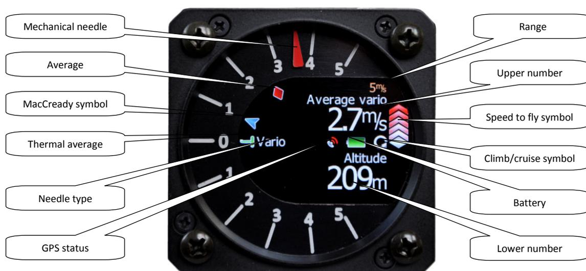
**Mechanical needle** displays vario, netto, relative or speed to fly value. It can be setup separately for climb mode or cruising mode. Printed scale can be chosen in range from -5 to 5 or from -10 to 10. Within software range can be set to 2.5, 5, 10m/s or 5, 10, 20kts or 500, 1000, 2000rpm.
