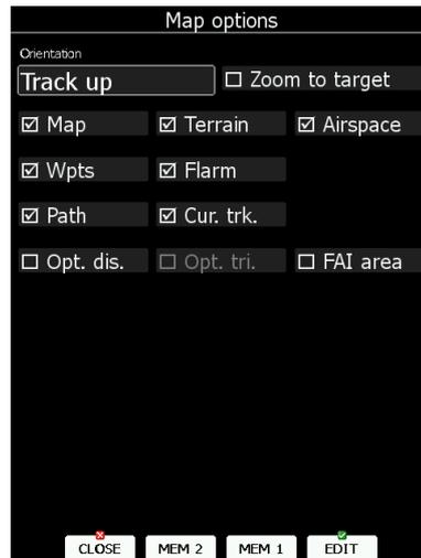
If **Zoom to target** is checked the zoom will be automatically adjusted so that the target point is always visible. Maximum zoom is 200 km and minimum zoom is 1 km. The check boxes will turn on or off the following items:
