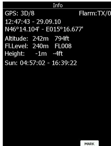
If you press the **MARK** button a new way point will be created with the current latitude, longitude and elevation based on the terrain database. The way point name is generated from the current date and time separated by the minus character and preceded by an underscore.
