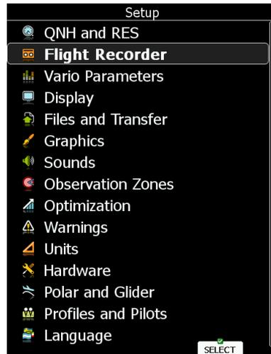
The setup menu is slightly different on the rear seat device as not all options are applicable. Items which are marked with an asterisk (\*) are available only in the front seat setup menu.
