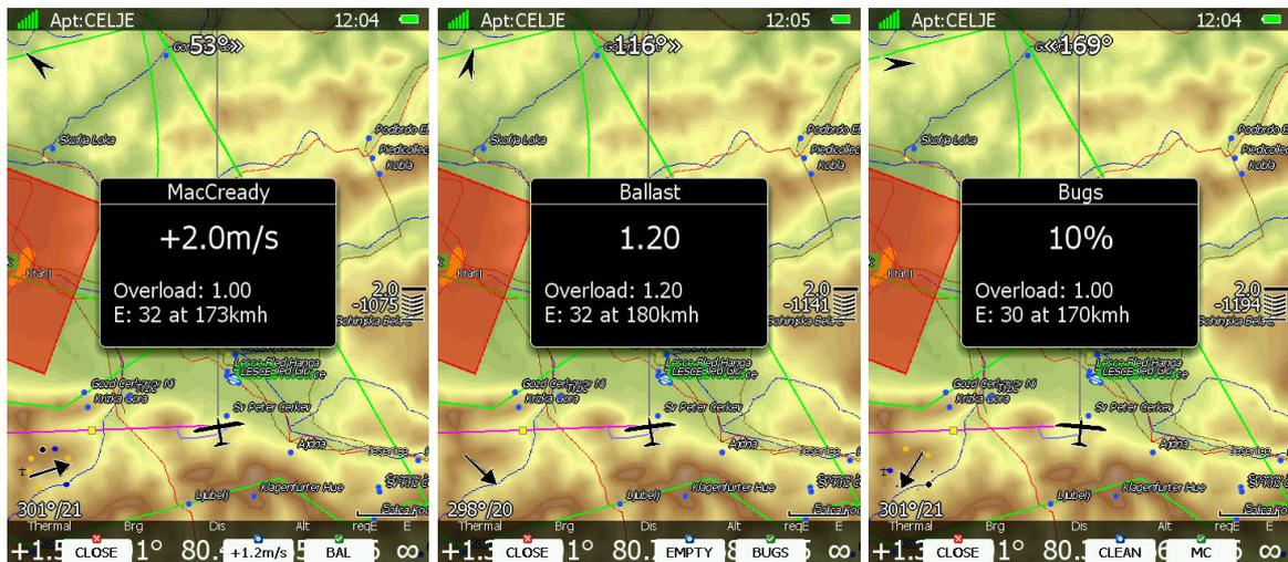
Use the lower-right knob to modify the MacCready setting. In the middle button there is a suggestion for the MacCready setting which is based on the last four thermals. Additionally to the selected MacCready value an overload factor is also shown together with the calculated glide ratio with corresponding speed.
