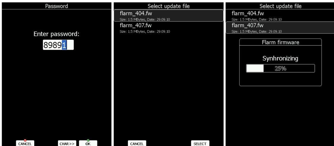
In case of a problem it is still possible to perform an update using FLARMtool and the serial connection. Please refer to an older LX8000 manual for the detailed procedure.
