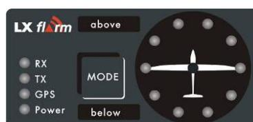
Radial positioned red/green LEDs define the direction to the near glider (top LED active means frontal collision risk). Two additional red/green light emitting diodes marked **above** and **below** inform about vertical position of the glider when close. The **Mode** button is used to control the unit. Four red/green LEDs indicate the Flarm status. The external display has two modes of operation:
