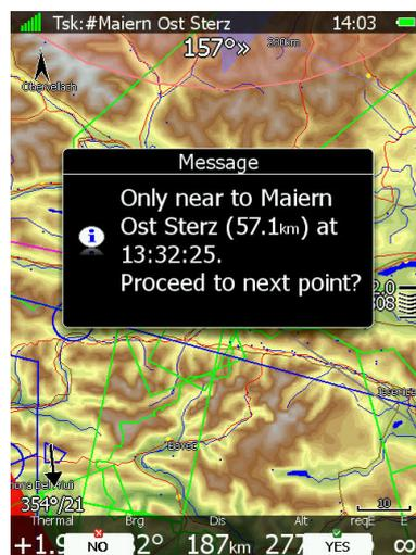
A message will appear. If you confirm this with **YES** the task will be advanced to the next turn point and it will recalculate the task taking the optimal fix as the task point.
