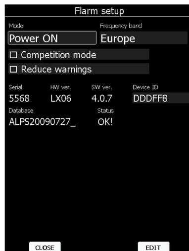
**Device ID** shows the Flarm unique ID, which is transmitted to other FLARMS. The Flarm status message is normally OK. In case of any errors or warning an error message will appear. The user can change the operation mode of Flarm unit, frequency and enable/disable competition mode.
