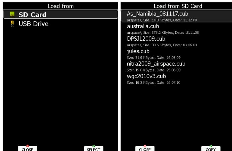
In next step the data source must be selected. A dialogue with a list of all available files will be opened. Press the COPY button to copy the selected file to the LX9000. The LX9000 will accept the following file formats:
