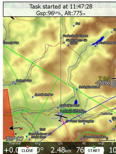
Ground speed and pressure altitude are also shown in the message. At the bottom two buttons are displayed. Use the **CLOSE** button if this was not a valid start and you want to remove the message from screen. If message is removed it will appear again next time you leave the start zone. If you press the **START** button navigation will be advanced to the first turning point.
