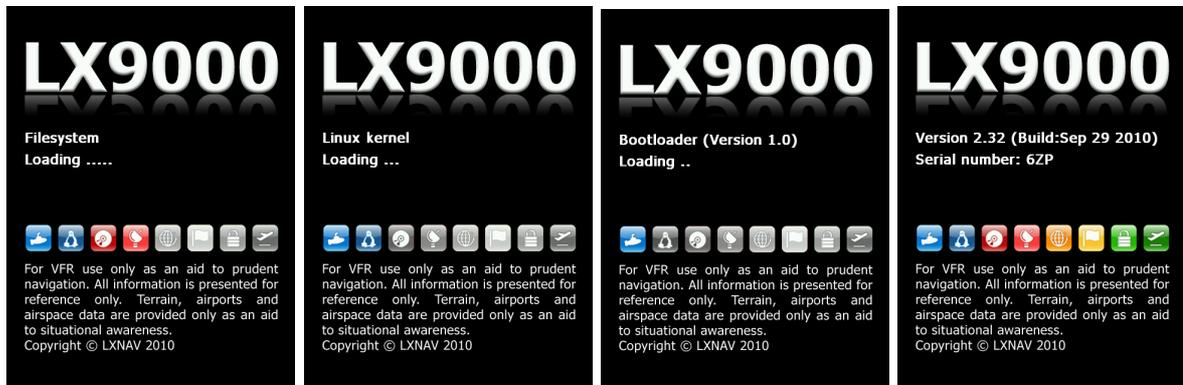
The boot procedure normally takes up to 20 seconds but in the case of a firmware update or system check it can take more time. The final boot screen displays information about the LX9000 firmware and the IGC serial number. When the boot procedure is completed the profile selection dialogue is shown. Please refer to Chapter 7.1 for more details about starting up the LX9000.
