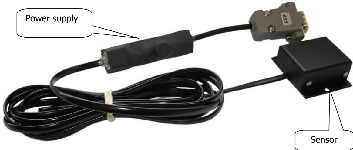
The compass module is an electronic compass device (magnetic field sensor) which was developed for the LX9000. The LX9000 recognises the compass module automatically when it is plugged into the RS485 bus. The only configuration settings needed are related to the compensation procedure. An indication that the compass module is connected is the appearance of raw data readings in the compass calibration page.
